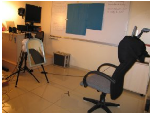
Figure 11: Acquisition setup. At the left 3D Digitizer, which is mounted on a tripod, is seen. A mirror, an LCD display and a 1000W halogen lamp are placed below, above and behind of it respectively. A seat is positioned about 1.5 meters away from the 3D Digitizer. On the floor, just below the seat, yellow straps are placed according to rotation angles.
